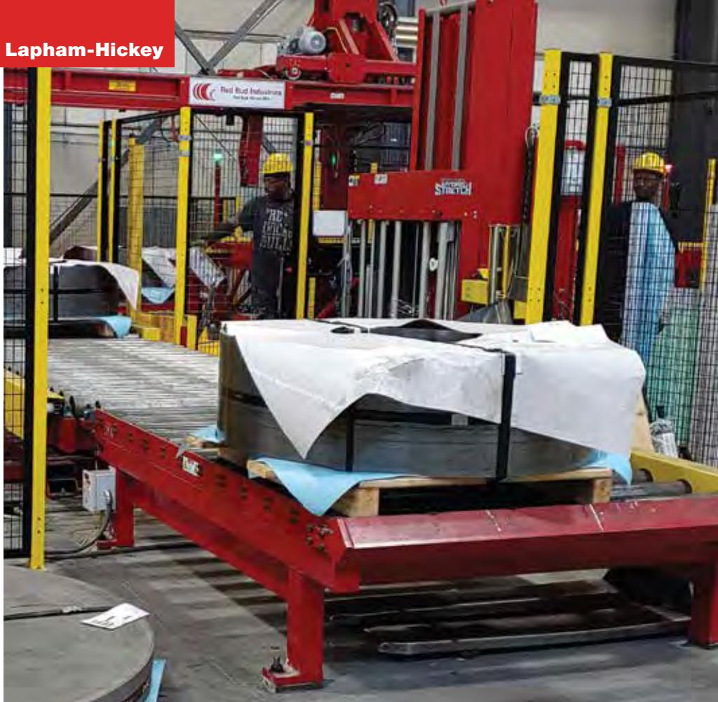
cycled down to a lazy Susan sortation table that can either move the material to be stretch-wrapped with an automated wrapper or can be taken off without banding. That feature truly increases production on the line, Karr says.
